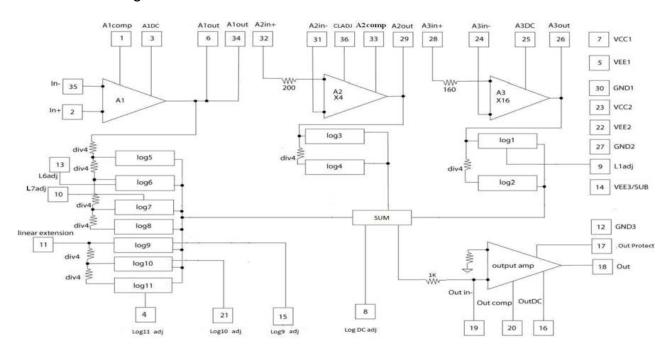
Note: for pinout A: Out Protect and Out are internally connected
