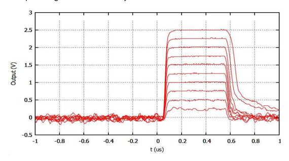
Notes: Pulse ladder has 5 dBm increments between rungs.
